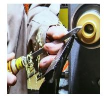
Once the thread cutting was complete the external dimension was sized and the collar piece was parted off.
