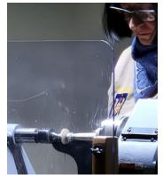
A spindle gouge was used to shape the handle and to form a bead immediately behind the collar disk
