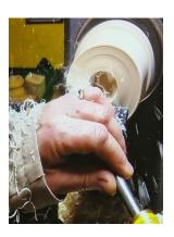
The hole was opened out to accept the internal threaded collar and it was glued in flush to the end. The box was then shaped using a spindle gouge taking care to not cut too short and into the hollowed box. It was then parted off.
