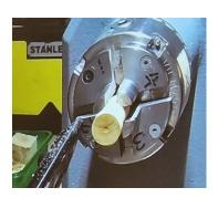
The lathe was slowed to approx 480 RPM, if this is not possible to dial up Carlyn recommends removing the chuck and slowing the lathe to the point where the chuck screw thread can be seen clearly rotating by eye and not a blur, i.e. observing each indvidual thread rotating and imagining it could screw relatively slowly into the machine by eye.
