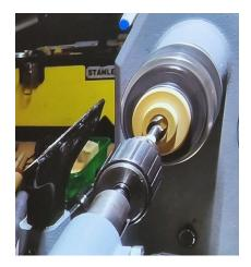
The required external diameter was opened up with a gouge and a hole smaller than the male threaded part was drilled through the entire piece, Carlyn reversed the piece to drill the opposite side, this allows the internal thread chasing tool clearance as it progresses into the piece.
